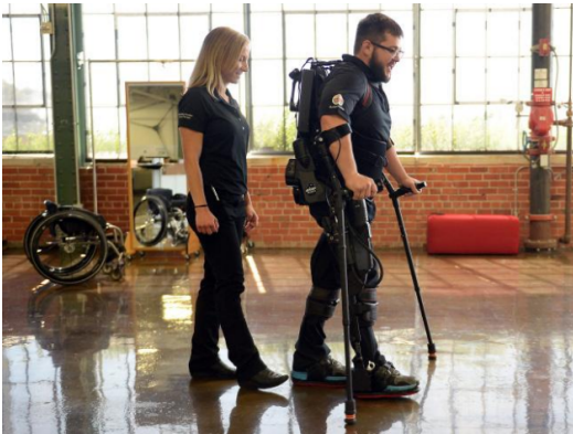
Fig. 3. Ekso Bionics exoskeleton, EksoGT™, used for data collection. We use two sets of its sensors in this study: hip and knee encoders to generate kinematics-based dynamical models using the NCD algorithm, and foot-mounted pressure sensors at the heel and toe to validate our models against ground-contact events after partitioning.
